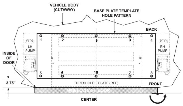
BASE PLATE TEMPLATE CLEARANCE FROM WHEEL-CHAIR DOOR (TOP VIEW, SIDE DOOR SHOWN) FIG. 27-1
